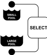
Press the **SELECT** Button after turning the power supply ON. The Select button activates the Large Pool / Small Pool cleaning cycles. When the cleaning cycle is running, the indicator light will stay lit on either Large Pool or Small Pool. (solid light)
